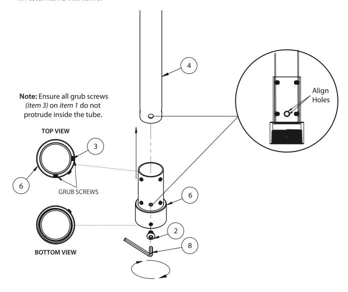
iii. Tighten the top 4 grub screws (item 3), securing the adaptor to the pole.
