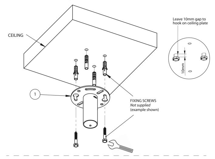
iv. Add remaining ceiling fixings and tighten all screws.
